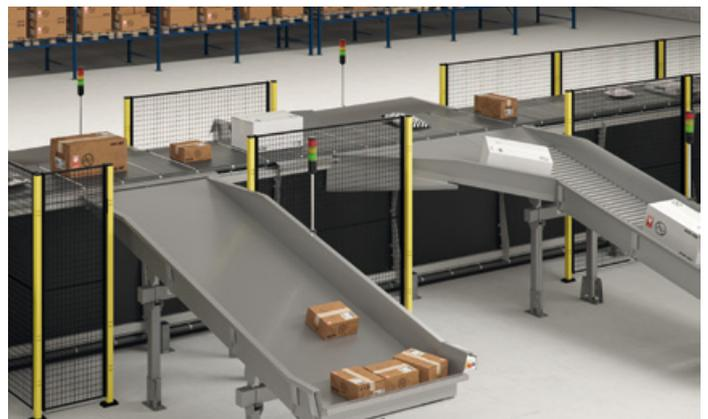
The simplicity in design allows for easy access to wear parts for fast replacement; for example easy maintenance access to each slat belt unit and drive unit without having to disassemble the chain of slat-belt units.
