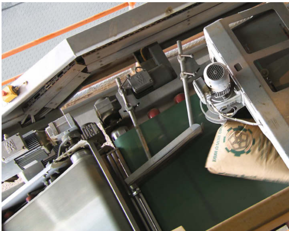
The bar-type turning device – as seen here in a BEUMER autopac® 3000 at Saudi Cement Company, Hofuf, Saudi Arabia – arranges the bags according to the chosen pattern.
