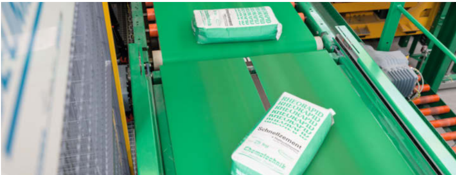
The twin-belt turning device brings the bags in the right direction.
