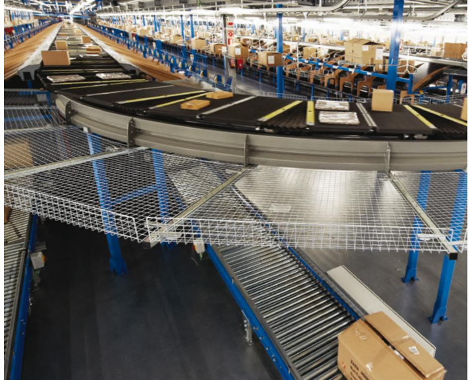
The flexibility lies in the sorter system using a one or two-belt per cart configuration that provides sorting capacity for up to four items per cart. Developed for manual and automatic induction on a cross-belt loop sorter, two items per belt gives a theoretically doubled capacity with discharge to left and right side (both items to same side or to either side).
