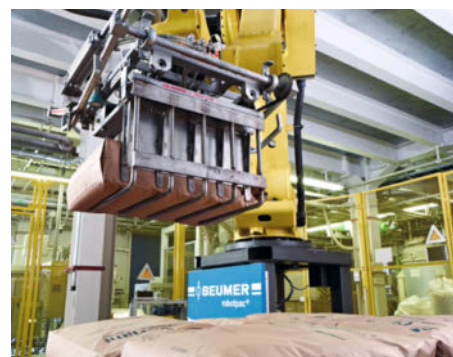
Fork gripper takes and stacks high-quality, bagged amide wax powder.
