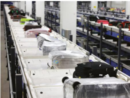
From the check-in areas in Terminals 1 and 2, conventional take-away conveyors transport the bags down to the apron level, where they are transferred to the tote-based CrisBag® system. This rapidly moves them via a tunnel to the BLC, where they are discharged onto conventional conveyors for security screening. At this point transfer bags are also merged into the flow.
