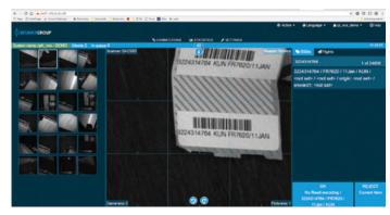
When installed, the camera images are run via an image pre-processor through to the image concentrator that interfaces with the Sort Allocation Controller (SAC). If installed on the existing ATR, the cameras can even run in parallel with the laser scanners. The process time for encoding each bag is fast enough to allow the bag to remain moving in the main system. The system can also make images available for attachment to various reports such as "no-read" reporting.
