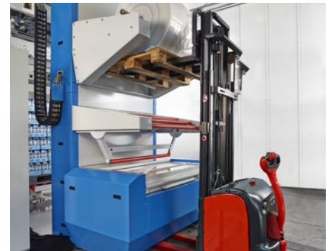
Fast exchange of the film roll with fork-lift trucks – simple control via BEUMER Group HMI
