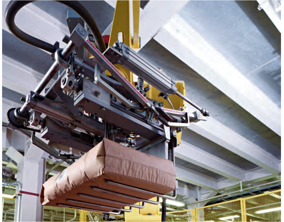
The BEUMER robotpac® enables reliable, secure and automatic palletising of a wide variety of materials.
