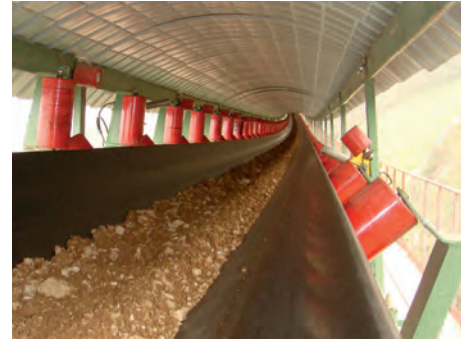
BEUMER troughed belt conveyor
