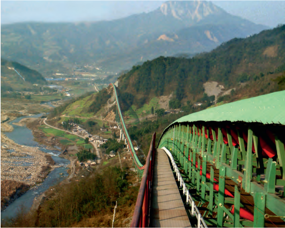
BEUMER belt conveyors also handle rough terrain with steep inclinations and tight curve radii.
