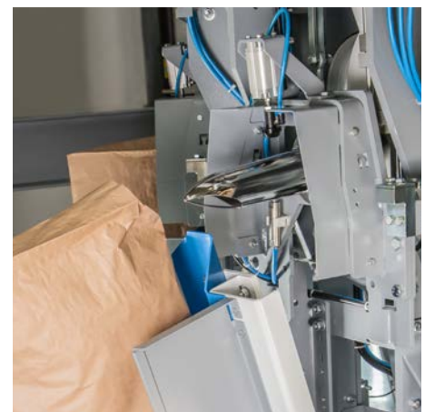
Optimised tilt frame for precise bag discharge
