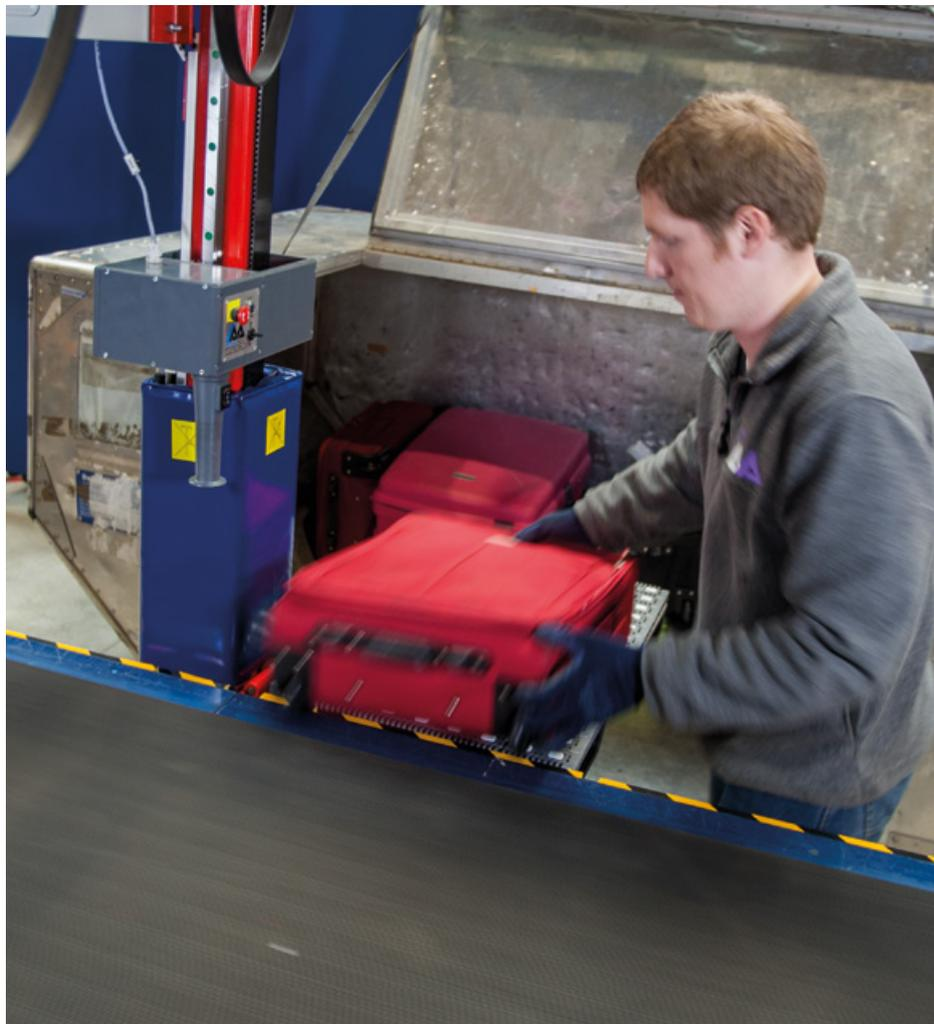
A throughput of around 10 seconds per loaded bag, combined with one-person operation, enables the Baggage Loader to optimise the baggage handling process, which allows staff to handle an increased number of bags, quickly and reliably. With easy integration into existing systems, the Baggage Loader is an affordable enhancement which can significantly improve the efficiency and the quality of the baggage handling process.
