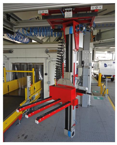
Easy integration into existing systems means that the Bag Forklift can be used to enhance the efficiency of virtually any baggage handling system.
