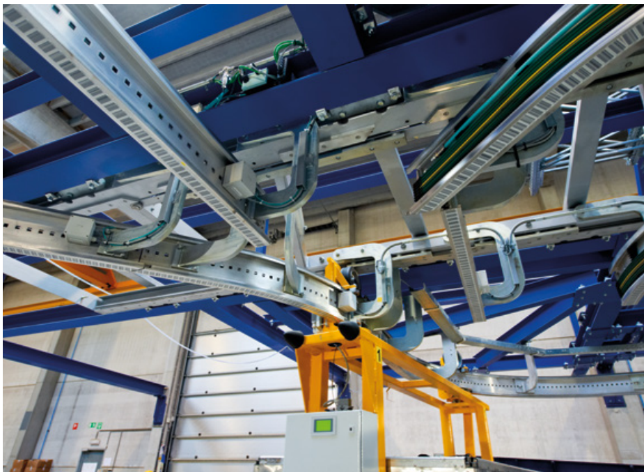
The management system can route carriers around interconnected loops
