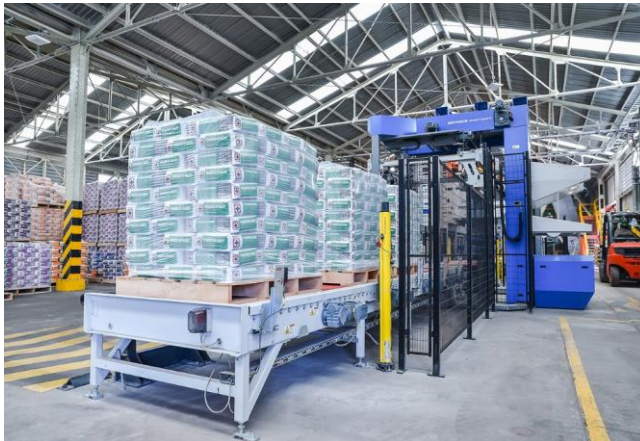
Image 9: BEUMER stretch hood A offers maximum load stability due to the combination of vertical and horizontal contracting forces of the film (Source: BEUMER Group)
