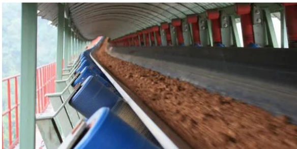
Image 2: Open troughed belt conveyors are used to transport bulk materials over long distances and through rough terrain (Source: BEUMER Group)
