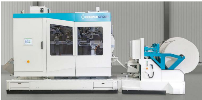
Image 6 The BEUMER Fillpac FFS forms bags from prefabricated PE tubular film, fills them and then automatically seals them (Source: BEUMER Group)
