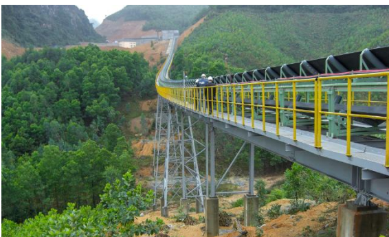
Image 6: Long distance conveyor GF1200x6532 (Source: BEUMER Group/FAM)
