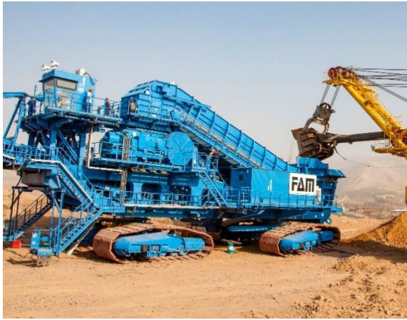
Image 7: Apron feeder AF2600x21 (Source: BEUMER Group/FAM)
