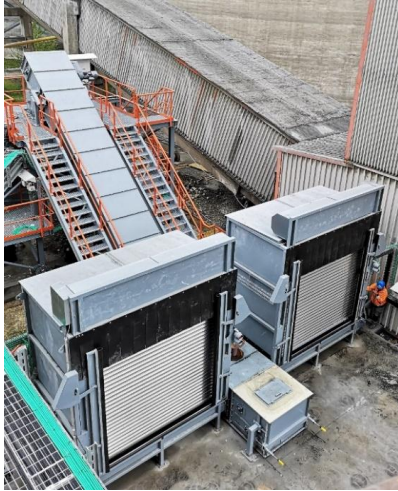
Image 3: BG OptiDock is a truck delivery station for alternative fuels. (Source: BEUMER Group)
