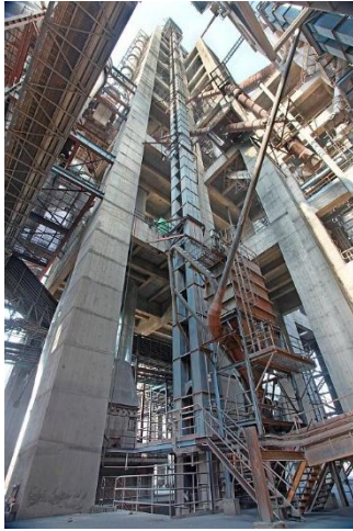
Image 1: BEUMER type HGBW belt bucket elevators convey the material to heights of up to 200 m and more (Source: BEUMER Group)
