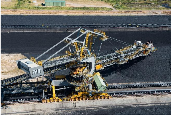
Image 4: Stacker-reclaimer STR6000/8000.60 (Source: BEUMER Group/FAM)
