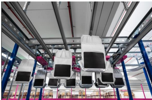
Image 4: BG Pouch System (Source: BEUMER Group)
