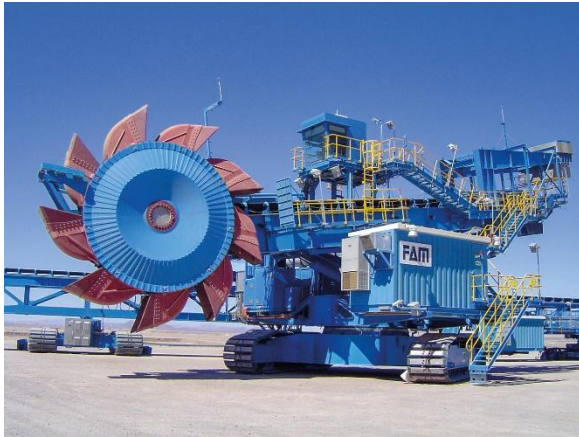
Image 1: Bucket wheel excavator SR500R4 compact type (Source: BEUMER Group/FAM)
