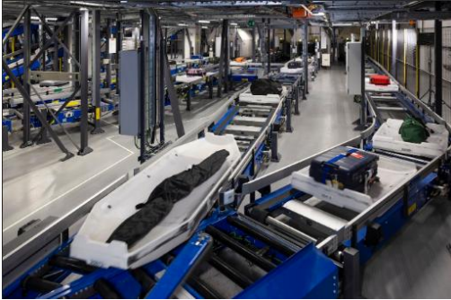
Image 2: CrisBag tote-based independent carrier system (Source: BEUMER Group)
