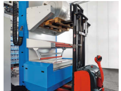
Fast exchange of the film roll with fork-lift trucks – simple control via BEUMER Group HMI
