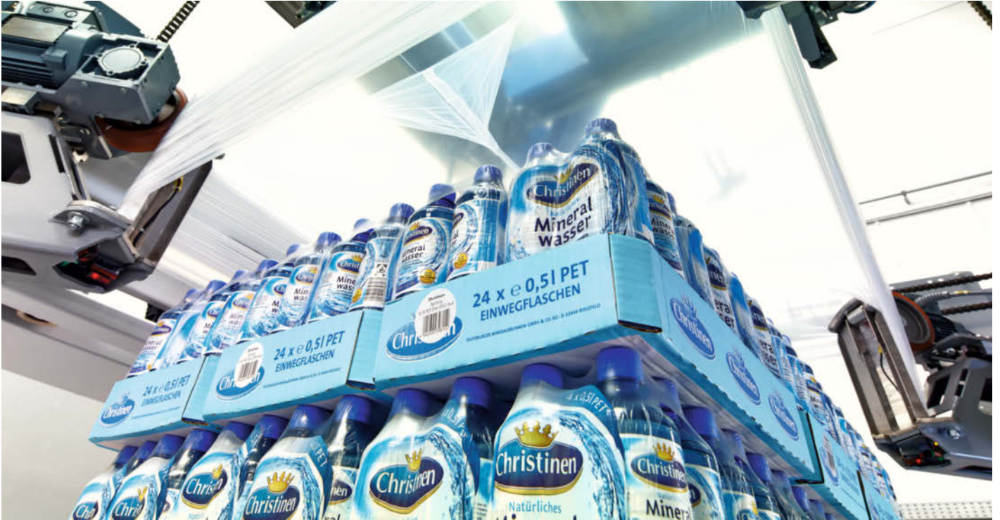
Spreading of the film hood and transfer to the crimping device
