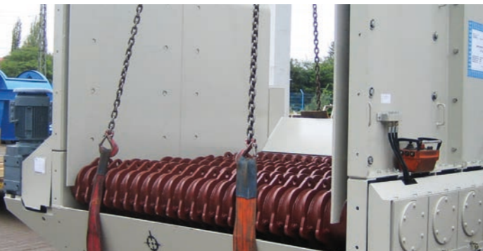
Roller screen RR2218, limestone 750 t/h, Kazakhstan
