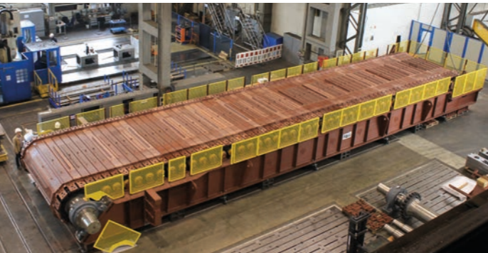
Apron feeder AF3400x22 heavy-duty type, oil sand 7260 t/h, Canada
