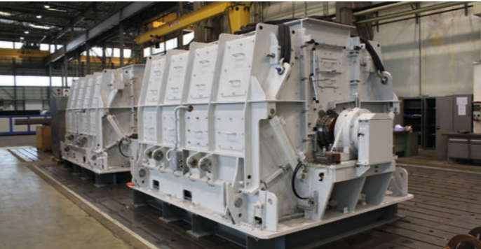
Reversible hammer mills PHM1628MVD, coal 650 t/h, China
