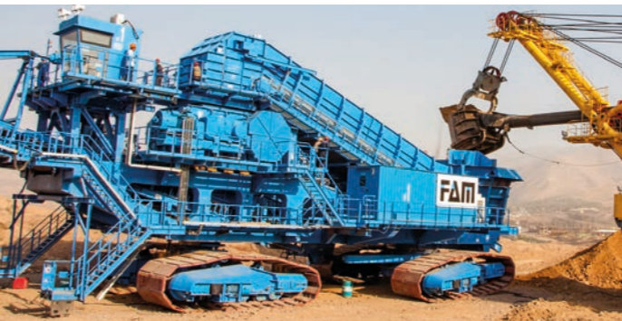
In-pit crushing system FZWB2025, on crawlers, overburden 5250 t/h, Uzbekistan
