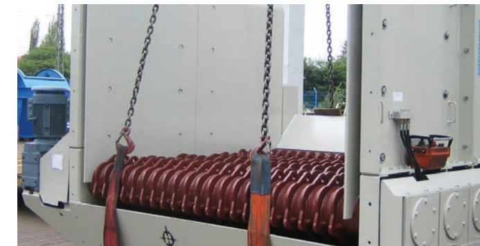
Rollenrost RR2218, Kalkstein 750 t/h, Kasachstan
