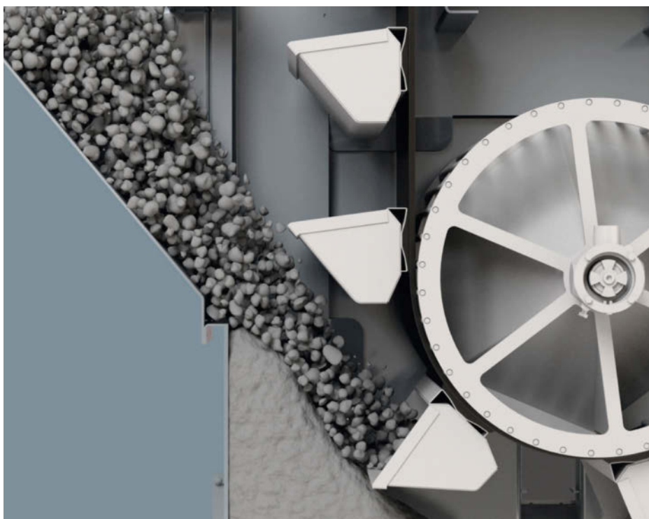
Optimised bucket design for minimum wear and long service life
