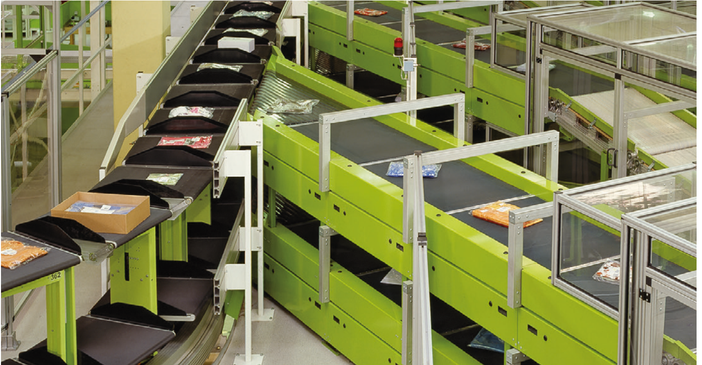
The BEUMER Belt Tray Sorter sorts and distributes any goods efficiently and gently
