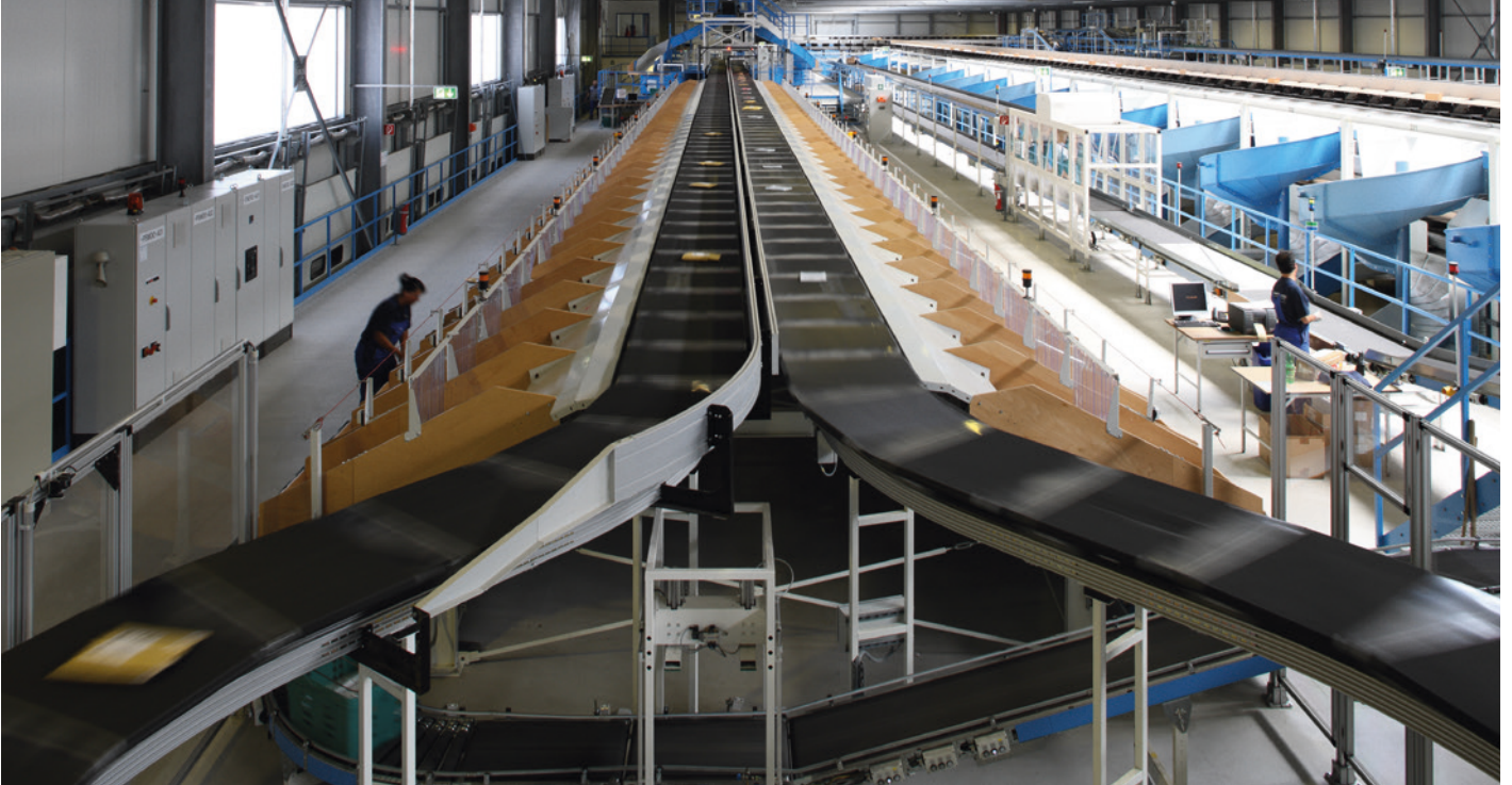
Sorter frame made of extruded aluminium profiles with integrated tracks
