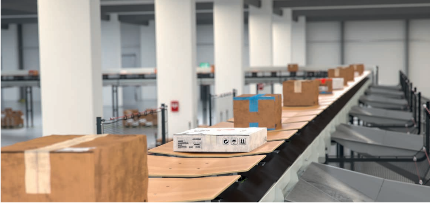
Safe transportation of parcels and goods with the BG Sorter ET tilt tray sorter
