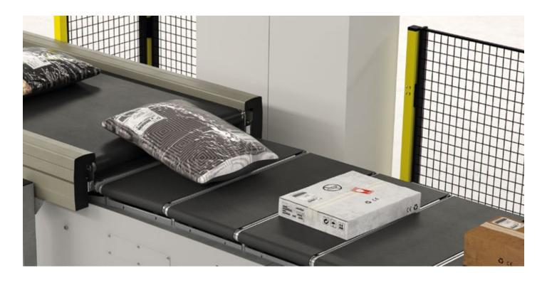
Get the best of both worlds: Our BG Line Sorter combines the simplicity of a line sorter with the exceptional handling capabilities of a high-speed cross-belt sorter in one system. The unique BEU-MER Group slat-belt technology expands the range of items that can be sorted. Setting new standards in the medium performance range.
