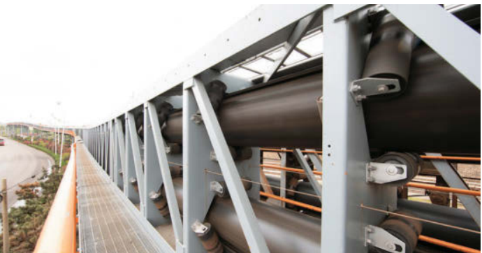
Pipe Conveyor for iron ore, China
