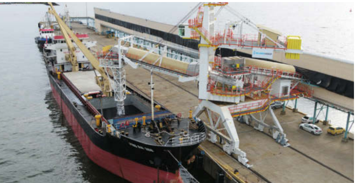
Ship loader for urea on Borneo, Malaysia
