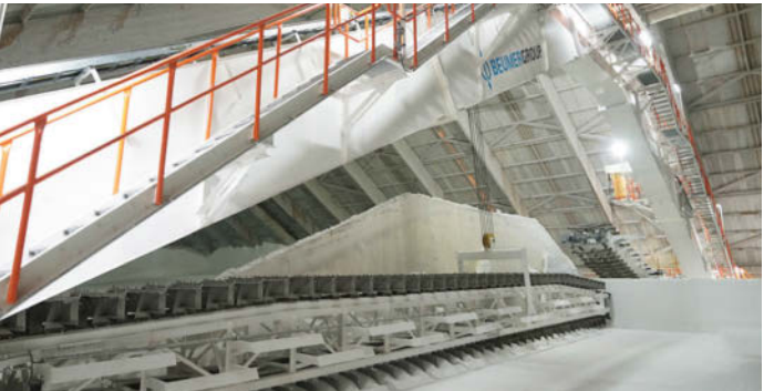
Double boom portal reclaimer for urea, Malaysia
