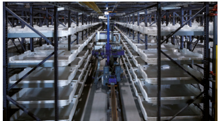
Dynamic, rack-based store for early bags as well as for the building of batches
