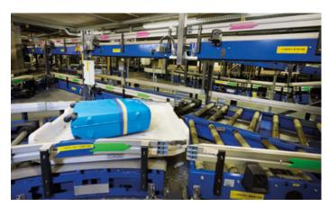
A tote system is, like the cart system, one bag per tote and one tote per logical section in the system. It is the simplest and most secure technology to control the individual bag.
