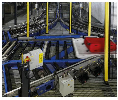
The system supports high capacity sortation and has redundant routes. With two sizes of totes, CrisBag handles standard bags as well as bags which are up to 1,400 mm long. To increase handling efficiency, standard and oversize bags are transported on the same track and at the same speed. This level of flexibility reduces the number of bags which are transported on the lines for oversize items.
