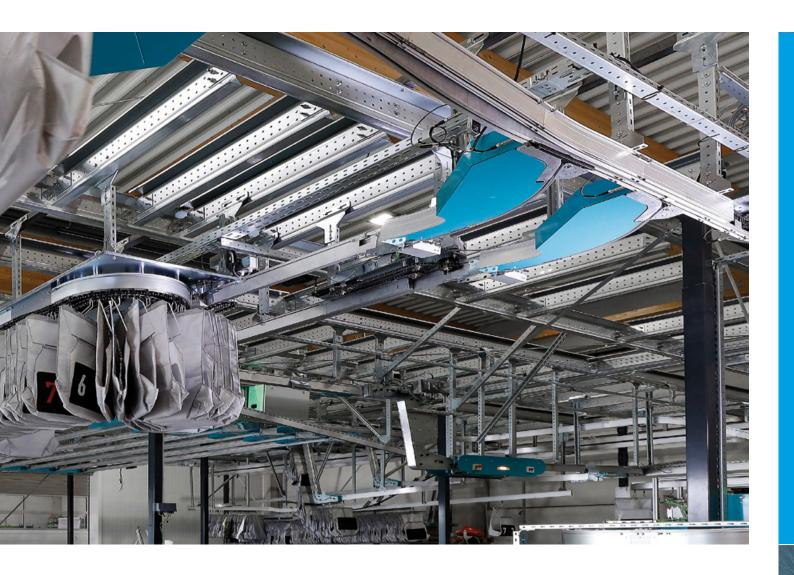
As a simplified logistics process, pouch sortation increases efficiency by reducing the number of times that each item is touched in the fulfilment or distribution centre. For returns handling, the need for less handling or touching is particularly critical.
