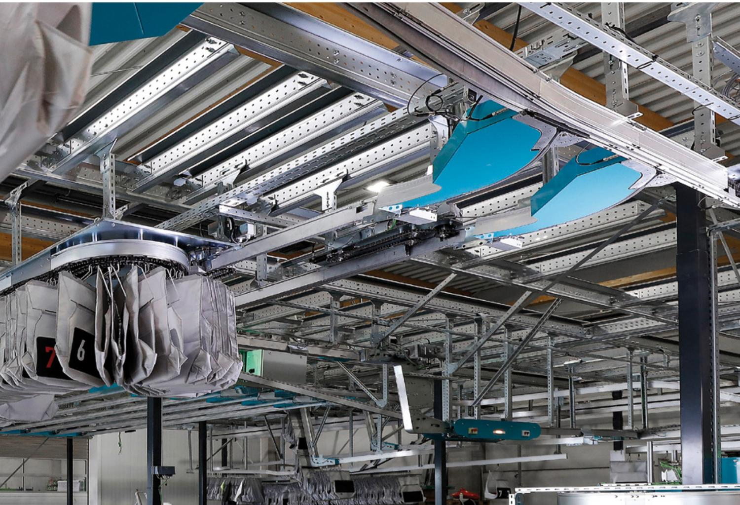
As a simplified logistics process, pouch sortation increases efficiency by reducing the number of times that each item is touched in the fulfilment or distribution centre. For returns handling, the need for less handling or touching is particularly critical.
