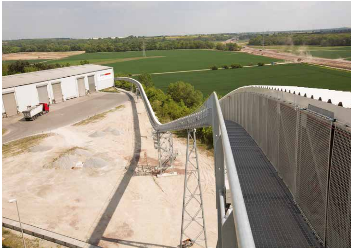
Horizontal curve overland conveyors and pipe conveyors can eliminate the need for transfer towers, saving capital costs and reducing maintenance.
