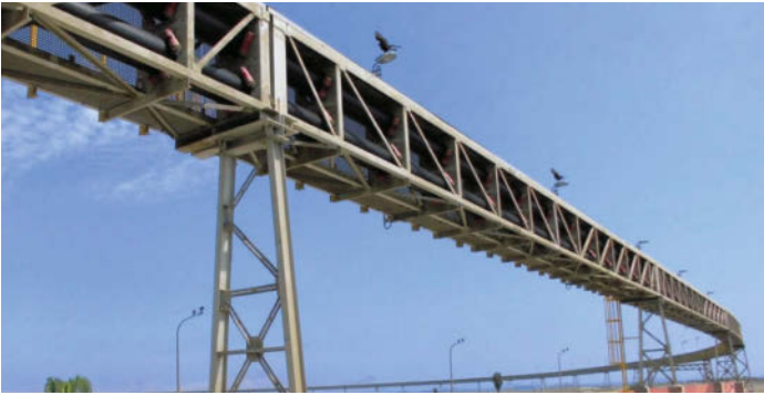
Pipe conveyor for copper concentrate in Collao, Peru
