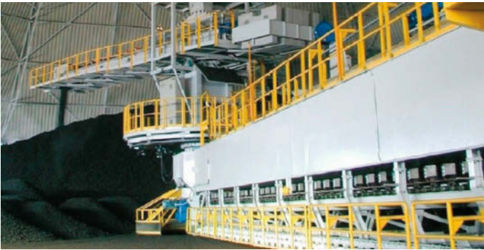
Circular Stockyard for coal in Slovakia (stacking/reclaiming)
