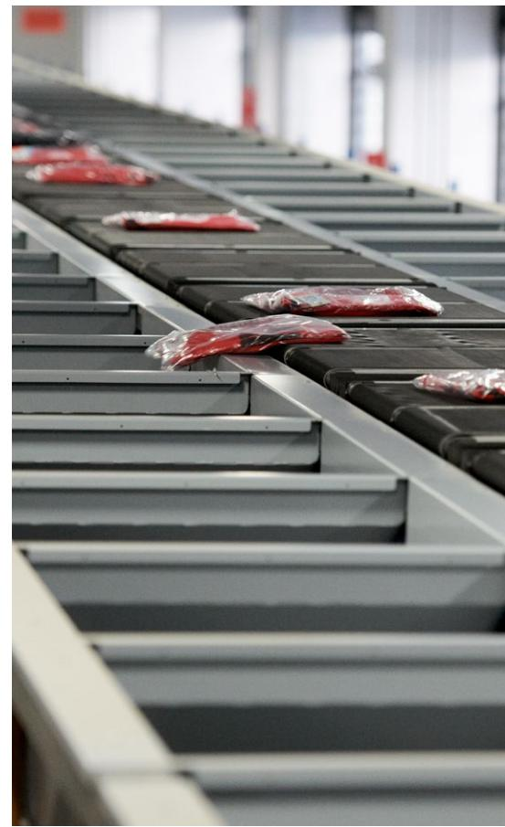
The BG Sorter CB is a cross-belt loop sorter that combines high throughput with exceptional handling flexibility, making it the ideal solution for parcel and distribution centers handling a wide variety of items, from small, delicate parcels to large, high-friction or rolling goods, effectively covering everything from a smartphone case to a refrigerator.
