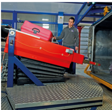
The Baggage Manipulator eliminates heavy lifting
