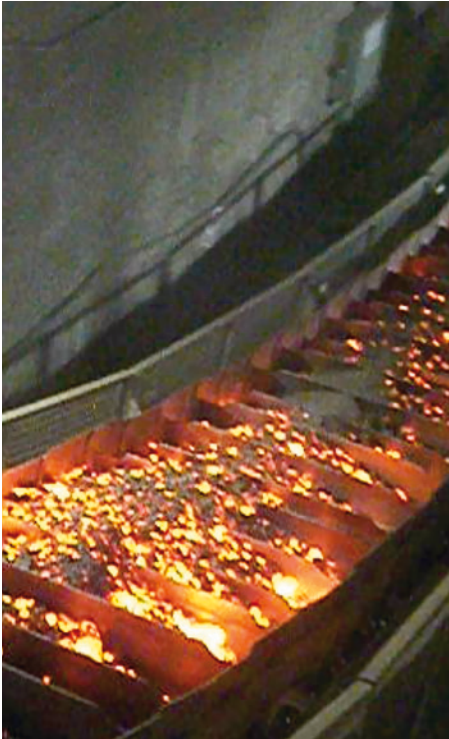
Transport of hot materials with temperatures of up to 600 °C and higher
