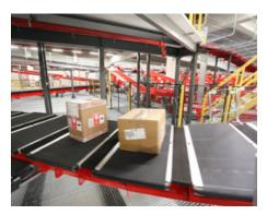
During the design phase it was suggested by BEUMER that basing the entire system on a series of crossbelt loop sorters would provide the optimum configuration by which DHL could achieve the highest item flexibility in terms of sizes and characteristics. Early in the design and development of the system, simulation proved that the operational capacity of the solution would be incredibly close to the theoretical capacity, something that is neither commonly nor easily achieved.
