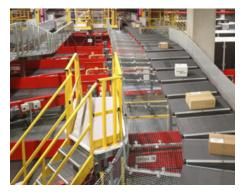
the sortation system was integrated with x-ray screening technology for security screening of all conveyable items. In addition to ensuring the capacity of the sortation system, the cross-belt loop sorters also ensure 100% track and trace of all items at all times during the automated sortation process. Everything was meticulously prepared to ensure a smooth transition for DHL's customers.
