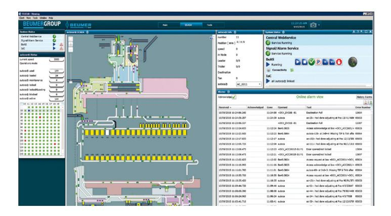
The upper level management system assigns tasks to the individual autoca and also includes a SCADA solution to monitor and operate the system in a -graphical, real-time overview. The SCADA shows the currecnt position of each autoca®, also when moving, as well as its technical and operational status. The system also offers the functionality to change flight data for loaded bags in the -autover® system, as well as extended statistical values in a graphical, real-time overview.
