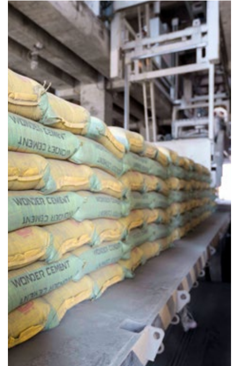
With layer calibration performed directly on the truck, the evenly piled bags ensure safe transport.
