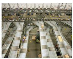
Coventry destination enters the hub via the upper sorter, it is automatically discharged to a conveyor and fed to the lower sorter to be taken to the chutes for other destinations.
