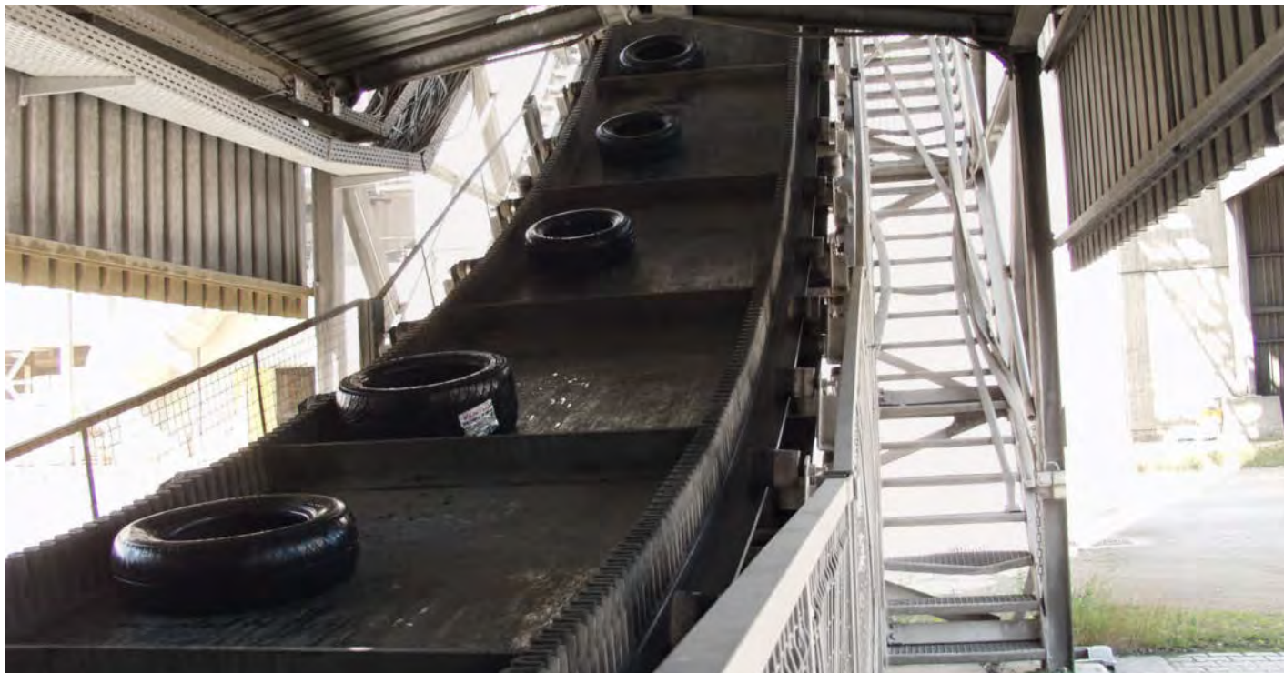
A flat belt conveyor with corrugated side walls lifts whole tires from the ground level to the point of feeding at the preheater.
