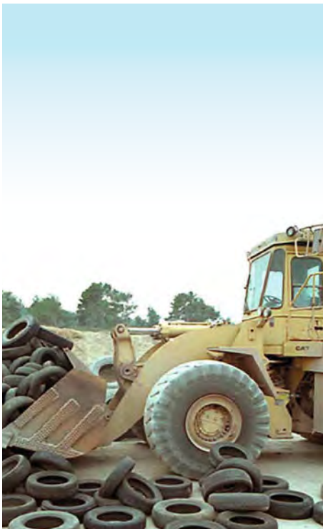
Whole tires can be fed easily by a wheel loader.
