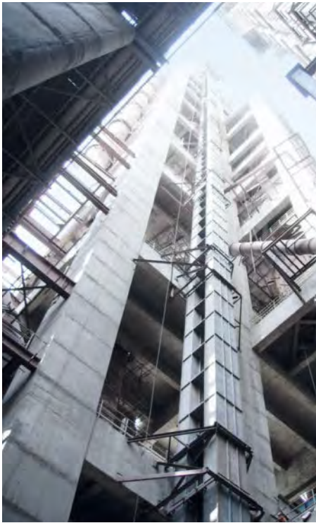
BEUMER high-performance belt bucket elevator
