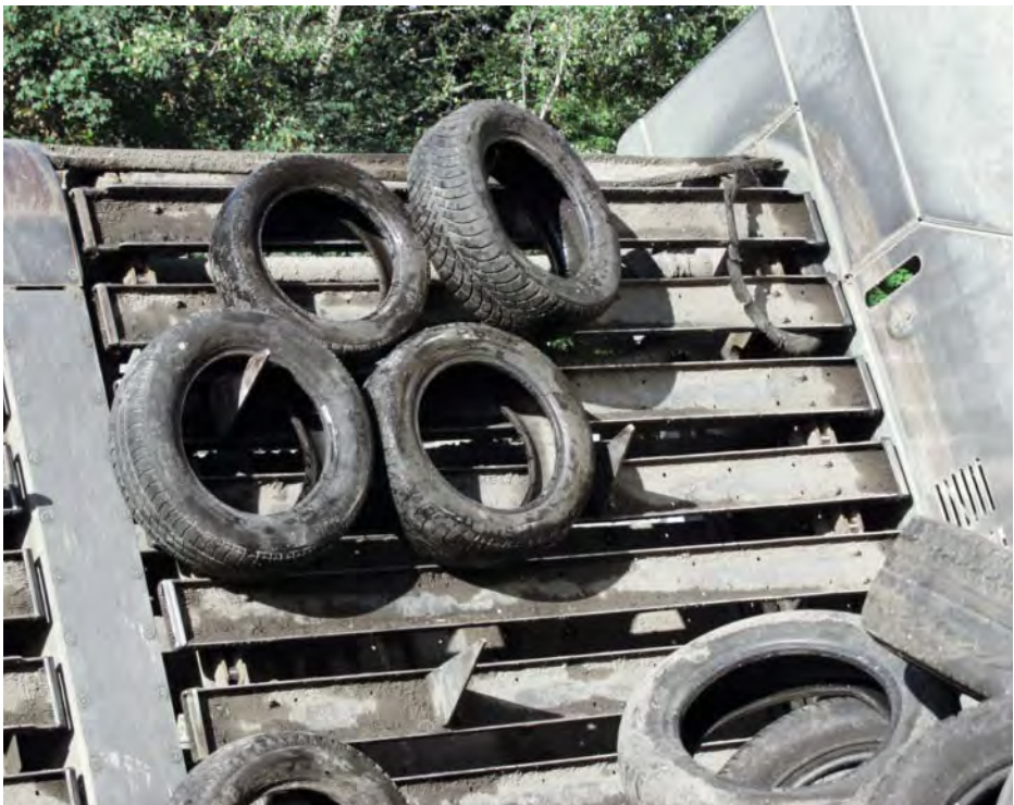
A hook lifter separates the whole tires for a controlled and continuous feeding.
