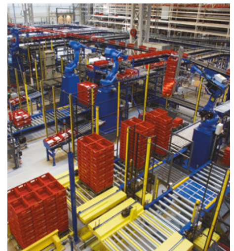
When a line of trays is ready for dispatch it is automatically released from storage and conveyed to robots for automated palletising.
