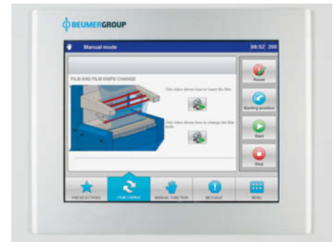
Assistance for the operator by means of video sequences, for example when changing the film roll on the BEUMER stretch hood®
