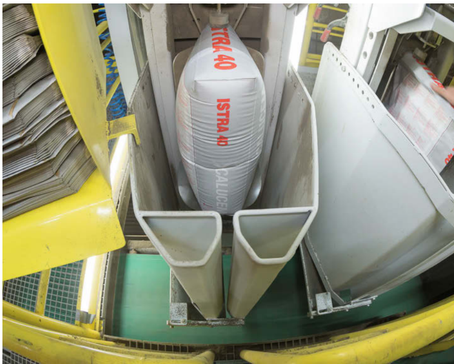
BEUMER fillpac® I with dust-proof enclosure
