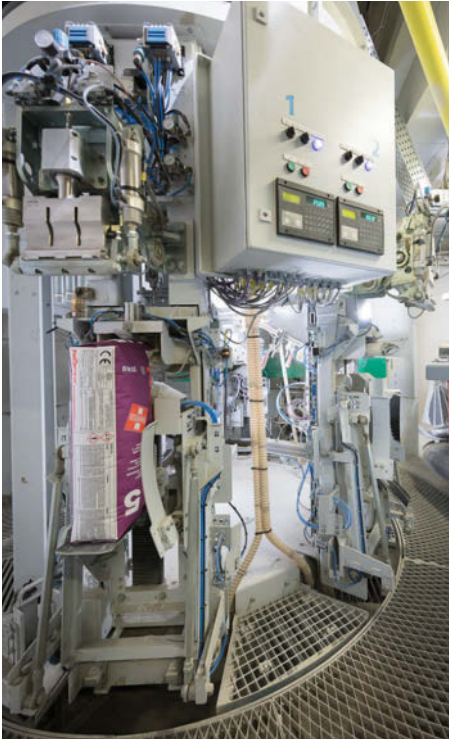
BEUMER fillpac® 6 spout air rotary filling machine with ultrasonic sealing
