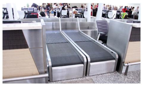
Twin passenger and operator displays simultaneously show the bag weight, total weight and the number of bags. Maintenance is simplified by a pull-out design along with the use of electrical plugs and sockets, which also eliminates incorrect connections, whilst the stainless steel design ensures an extended operational life.
