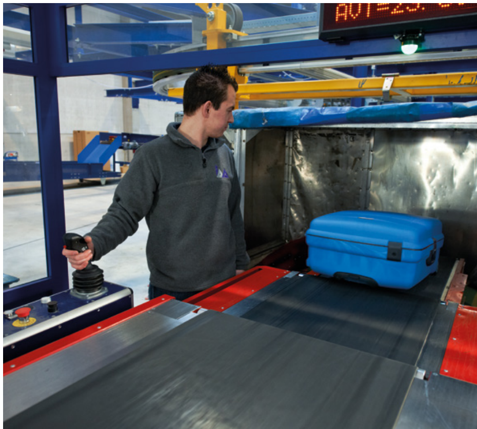
Each bag gently slides off the ramp into its position in the ULD
