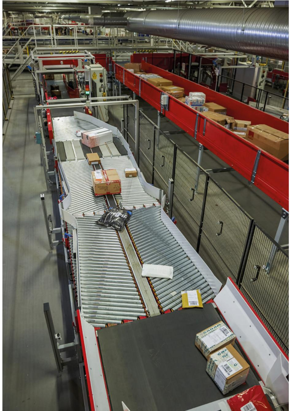
minimises wear and tear to enable the Automatic Parcel Singulator to achieve very low maintenance levels.
