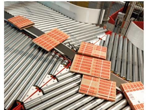
As a fully automated system, the Automatic Parcel Singulator minimises the need for manual handling and supervision during normal operation.
