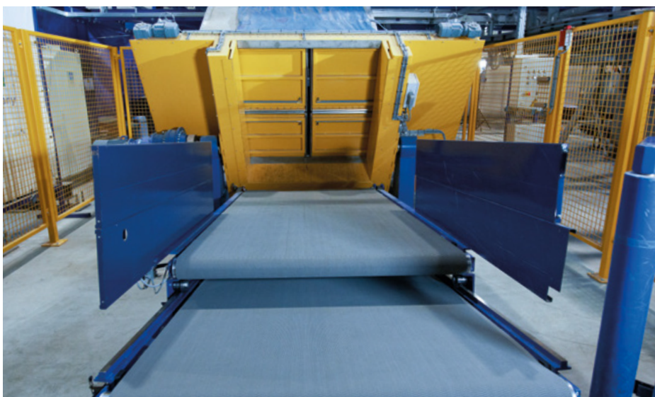
The unloader automatically tips each ULD twice to ensure that every bag is transferred to the conveyor
