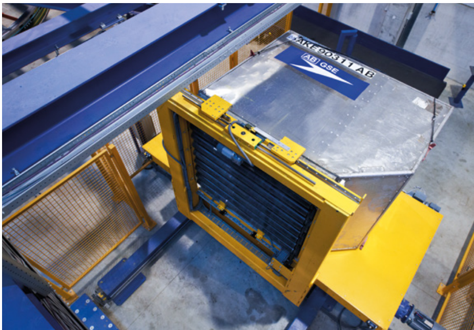
The ULD is automatically positioned into the Automated Container Unloader
