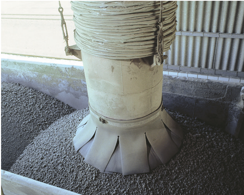
Fast, dust-reduced bulk material loading
